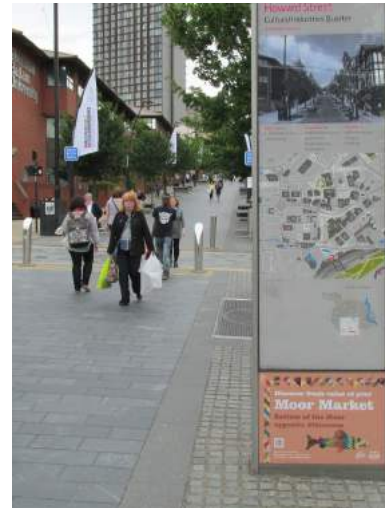
Figure 3.9: Wayfinding elements used in combination - wayfinding map, banners and unified paving to identify key routes
